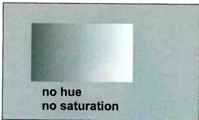
Figure 7. As more light of all wavelengths is added to light of a single wavelength (a single color), eventually the color reaches zero saturation, which is white light.
