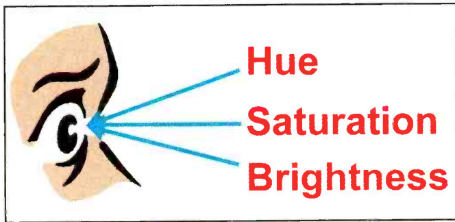
Figure 5. The human eye/brain system responds to three different characteristics of light: hue, saturation, and brightness.
